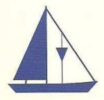
Sailing Vessels when under power One black cone, point down
